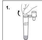
Remove the foil from the top of the extraction buffer tube.
